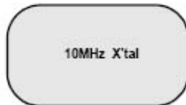
⑥ 10MHz X'tal IC001 PIN 50 (OSC)
