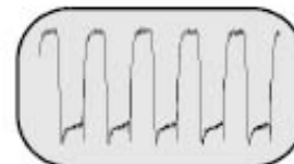
⑮ 2.88 Vp-p IC801 PIN 7
