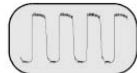
⑯ 114 Vp-p Q501 Colector
