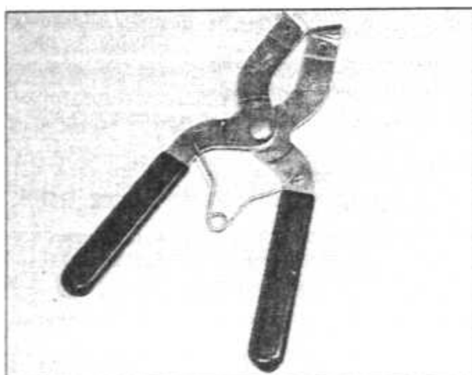
Piston ring removal/installation tool
