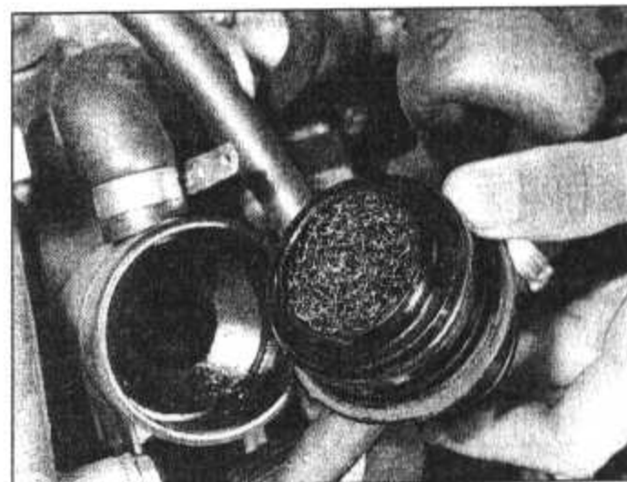
2.10 Oil filler cap showing filter mesh (OHC engine shown)
