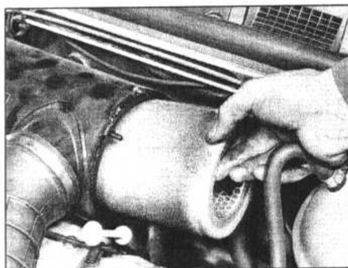
18.3 Removing the filter element
