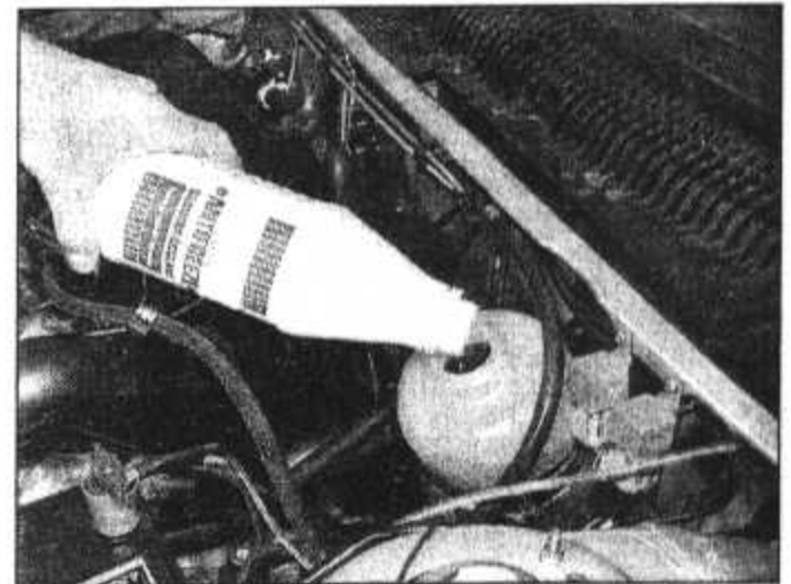
6.20 Topping-up the expansion tank
