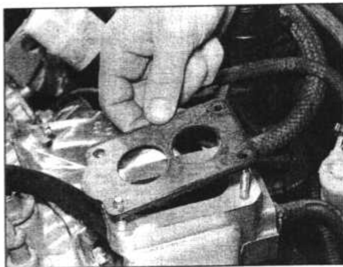
7.24 Removing carburettor spacer
