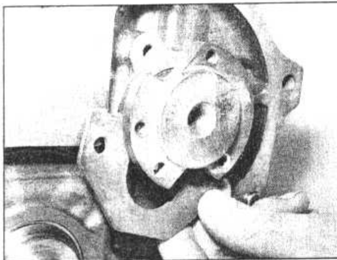
42.2A Locate the camshaft thrust plate ...
