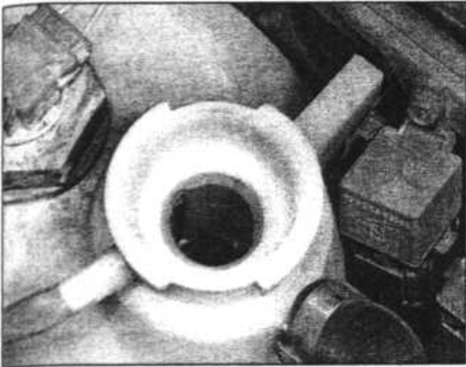
6.3 Coolant expansion tank level guide tube
