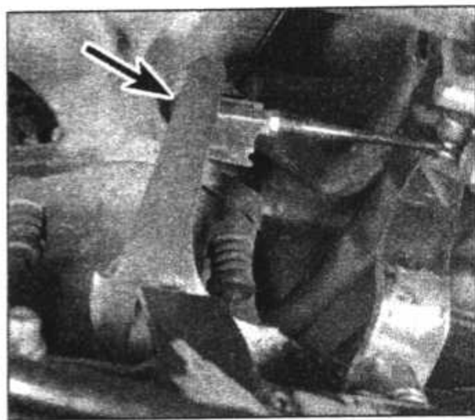
5.7 Gear selector rod viewed from underneath. Note the heatshield (arrowed)
