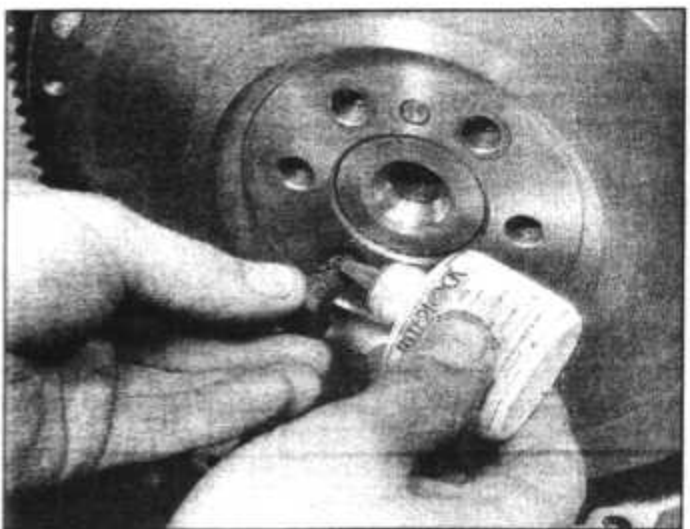
5.129A Apply locking fluid to the flywheel bolts...
