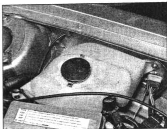
30.1A Windscreen washer reservoir and pump unit (arrowed) - SRi model
