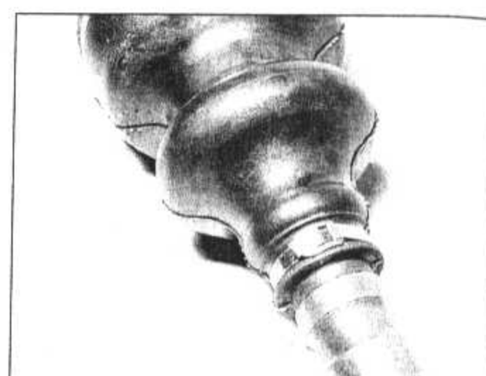
15.15B Bellows clip correctly fitted
