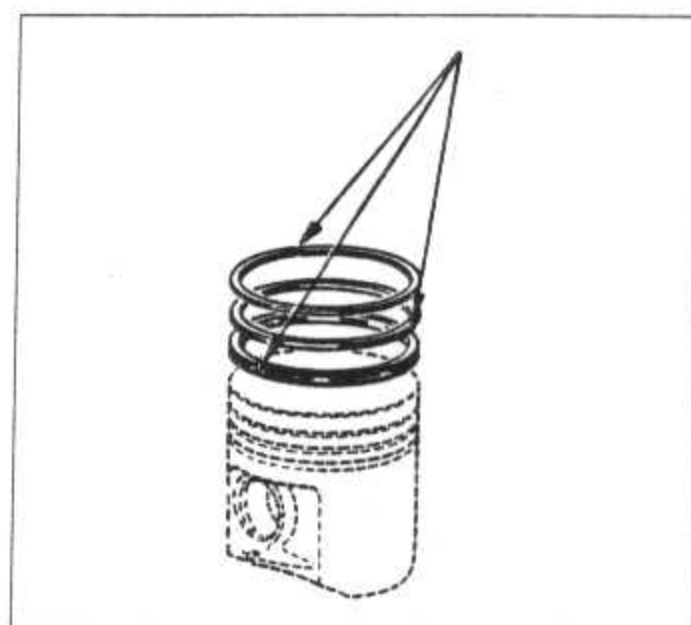
Fig. 1.18 Space the ring gaps when fitted as indicated (Sec 40)
