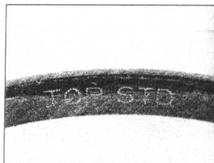
40.5 Orientation and size mark on the top piston ring
