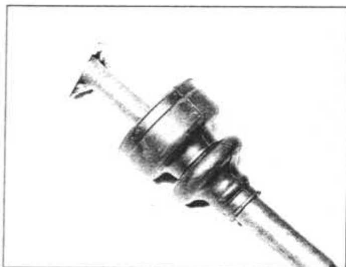
15.12 Inner joint bellows located on the driveshaft
