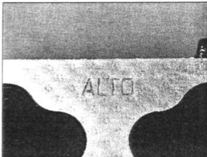
47.4A Position cylinder head gasket with ALTO marking uppermost
