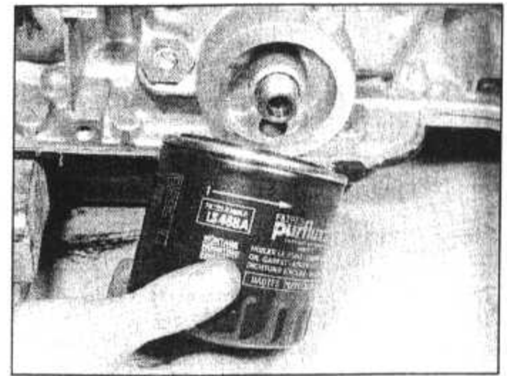
5.59 Removing the oil filter
