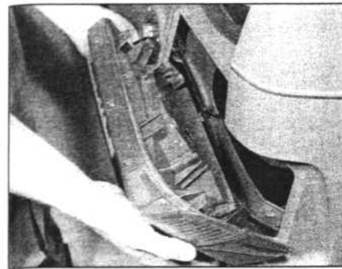
16.18 Rear combination light lens removal
