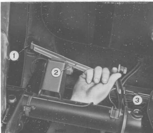
Checking the distance between friction bar eye and bumper mounting plane.
