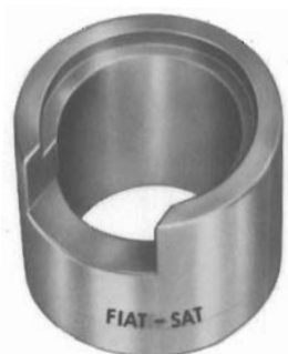
A. 74281 Adapters for mounting „Hiperbloc“ bushings in shock-absorbers (to be done on a press).
