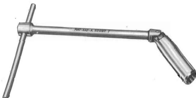
A.50087 Spark plug spanner (to be used on the vehicle).
