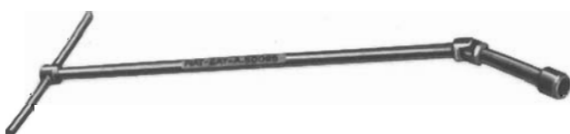
A.50095 Articulated spanner (13 mm) for starter motor dismounting and reassembly (on the vehicle).
