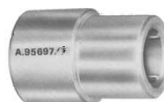
A.95697/7 Socket used in conjunction with A.95697 dynamometer for checking the torque required for turning steering gear drive shaft with worm.
