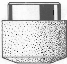
Grinding wheel with working face at 20° angle.
