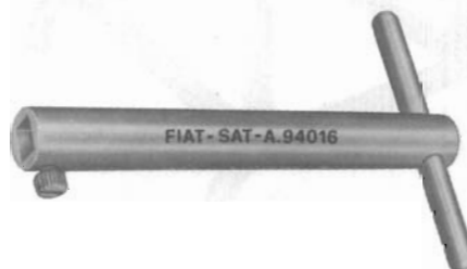
A.94016 Handle for plug seat countersink.
