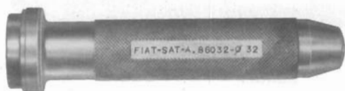
A.86032 Ø 32 mm mandrel for inserting cylinder block plugs.
