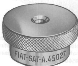
A.45027 Bushing for stripping bearing inner race from differential carrier (to be used together with A.40005/002/302/400).
