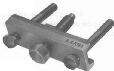
A. 47085 Puller for front wheel hub.
