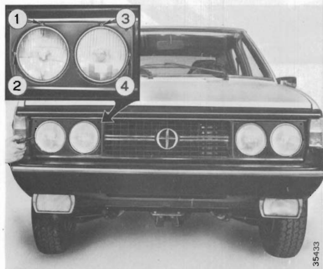
Headlight adjusting screws.
