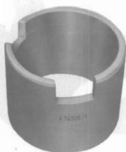
A.74108/1 Bushing for stripping, on a press, the bearing and locating ring from drive shaft (to be used with A.74108 half-rings).
