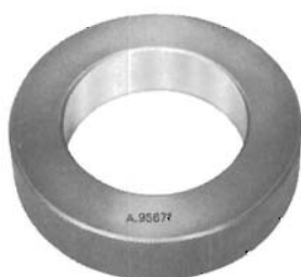
A.95671 Ø 72 mm ring gauge for calibration of A.95687 cylinder gauge to check cylinder bores of 1300 engine.
