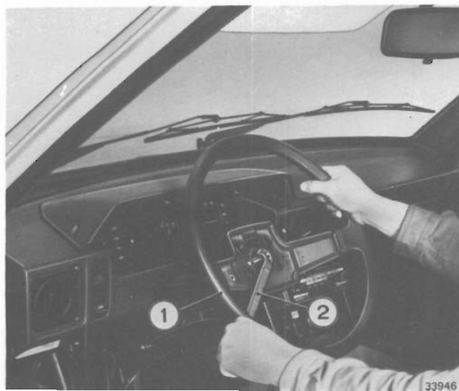
Unscrewing steering wheel to steering column fastening nut.
