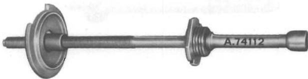
A. 74112 Fixture for front suspension helical spring compression.
