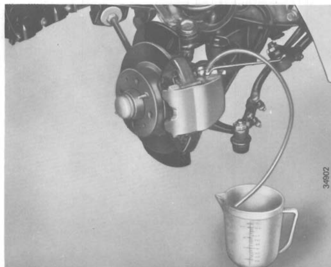
Bleeding the left-hand front wheel brake.
