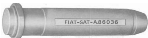
A.86036 Ø 36 mm mandrel for inserting cylinder block plugs.
