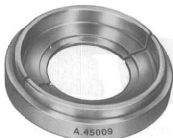
A.45009 Bushing for stripping bearing inner race from final drive pinion (operation carried out on a press).
