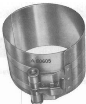
A.60605 Spring band for inserting nominal size and oversize pistons in cylinder bores.
