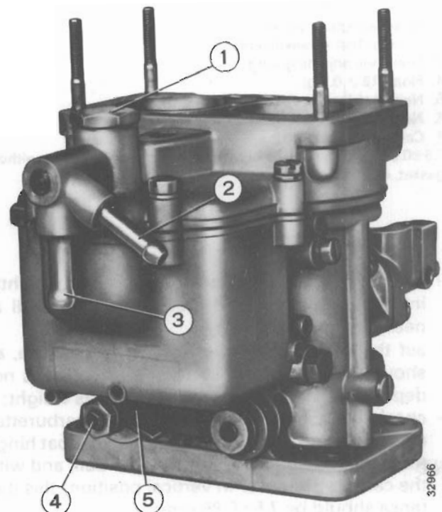
View of carburettor from the side of acceleration pump and excess fuel recycling connection.
