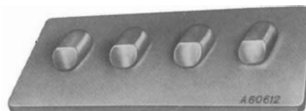
A.60612 Cylinder head support stand for valve installation and removal.
