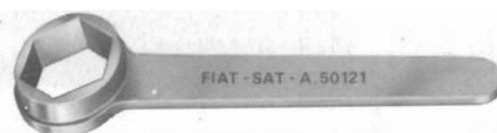
A.50121 Box spanner for pulley to crankshaft clamping nut.
