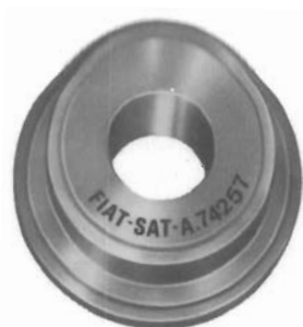
A. 74257 Mandrel for mounting front wheel bearing outer race.
