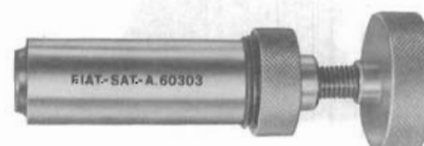
A.60303 Device for inserting gudgeon pin retaining clips.
