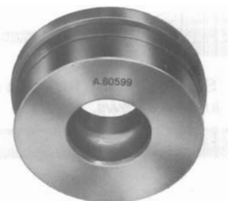
A.60599 Ring for fitting and removal of rear camshaft bearing (to be used with A.74365 ).
