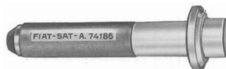
A.74186 Punch for installation of worm bearing outer race.
