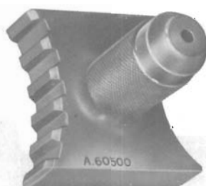
A.60500 Block for immobilizing the camshaft pulley while unscrewing the clamping screw.
