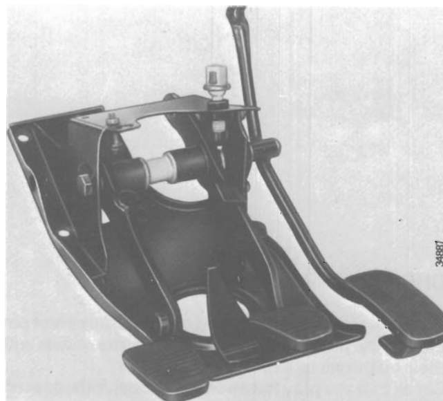
View of pedal bracket assembly.
