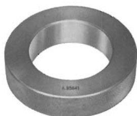
A.95641 Ø 77 mm ring gauge for calibration of A.95687 cylinder gauge to check cylinder bores of 1500 engine.
