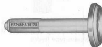
A.70173 Punch for mounting pinion rear bearing outer race in rear axle housing.
