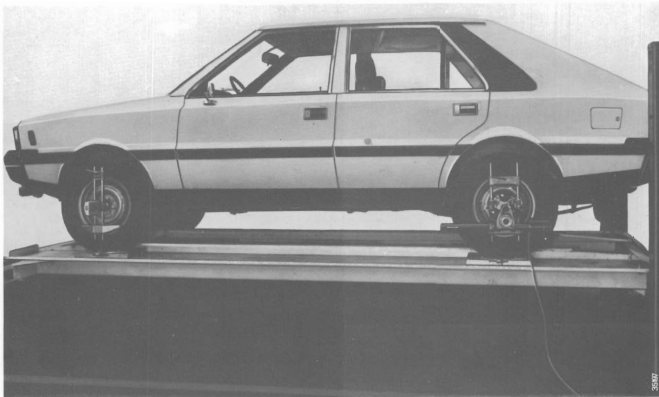
Checking front and rear wheel setting.
