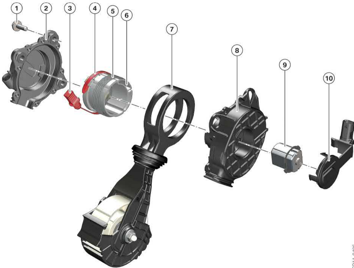
N13 engine, friction gear servodrive - exploded view
