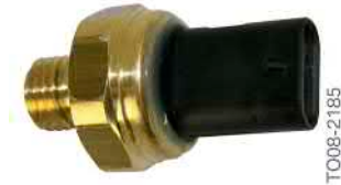
N13 engine, oil pressure sensor
