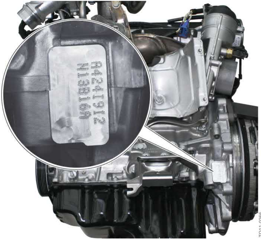
N13 engine, engine identification and engine number
