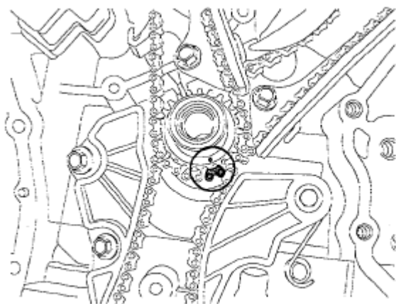
Fig. 75: Matching Timing Mark With Sprockets Courtesy of KIA MOTORS AMERICA, INC.
