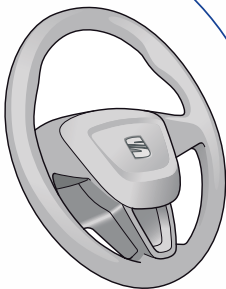
Driver's front airbag detonator, N95
