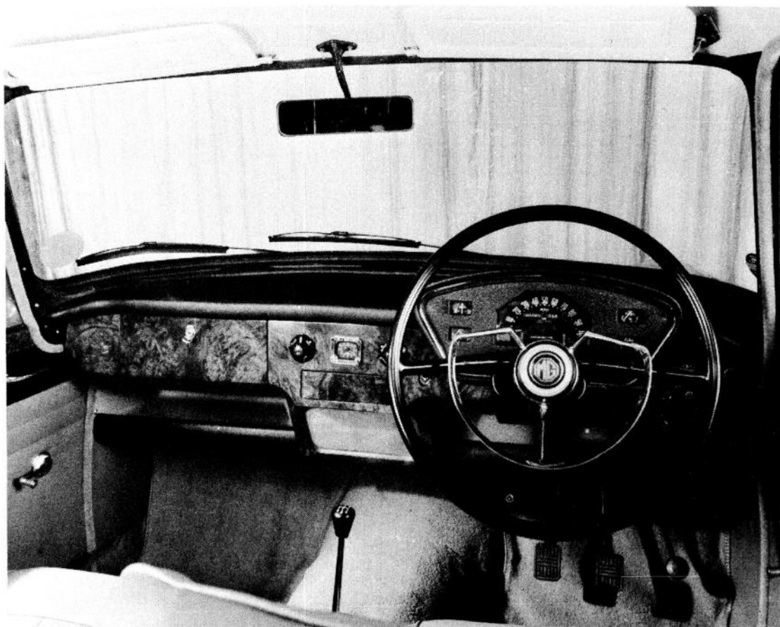
Fig. 10. MG 'Magnette' instruments and controls
