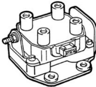
The windings are covered by a pressed plastic container and are insulated through immersion in an epoxide resin and quartz compound which gives them exceptional dielectric, mechanical and thermal properties enabling them to withstand high temperatures.
