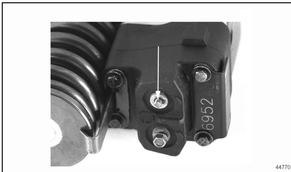
Figure 6-7 Broken Solenoid Terminal Screw Failure
