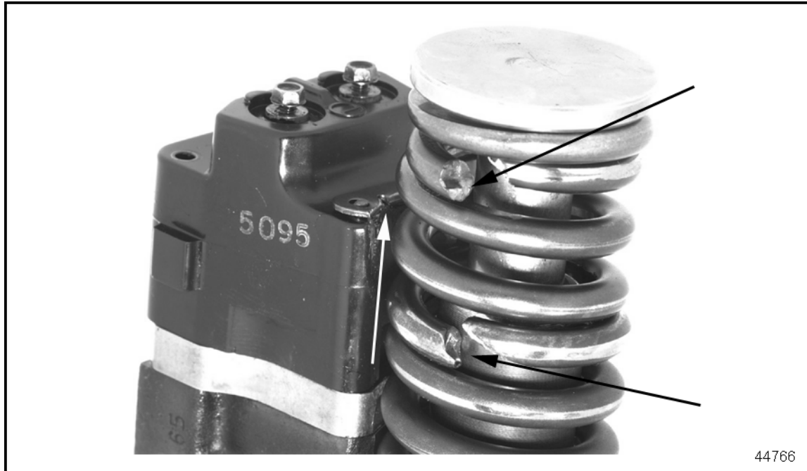
Figure 6-3 Broken Injector Follower Spring And Damaged Stator With Broken Stator Screws Failure
