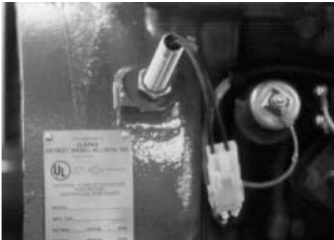
Fig. 9 - Magnetic Pickup
