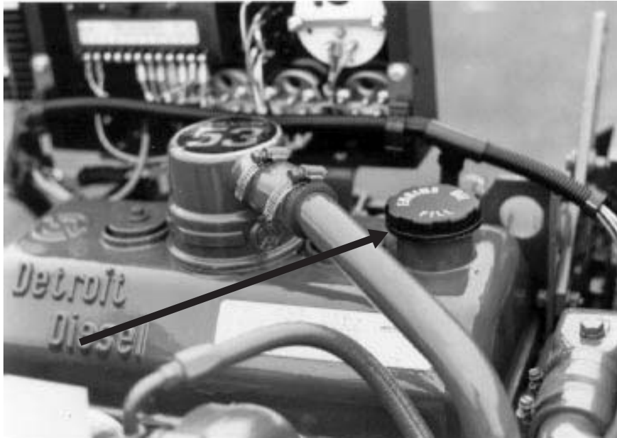
Fig. 5 - Typical Oil Fill Location
