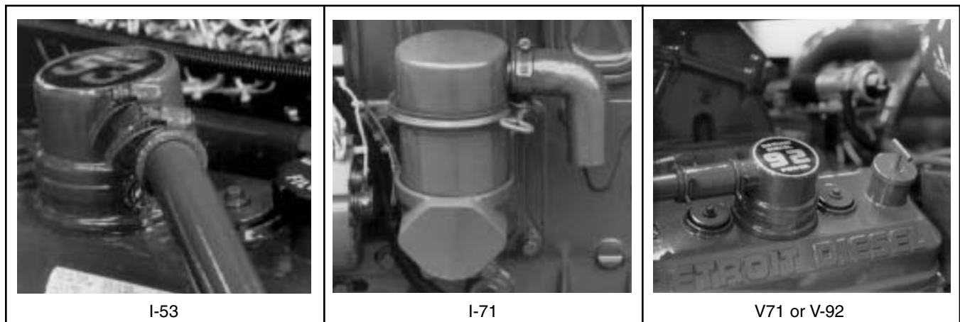
Figure 2 - Crankcase Ventilation
