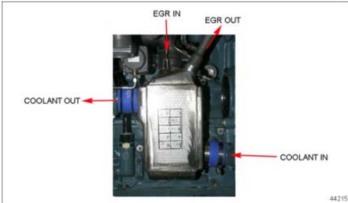
**Figure 2-10 EGR Cooler (Bar and Fin Design)**
