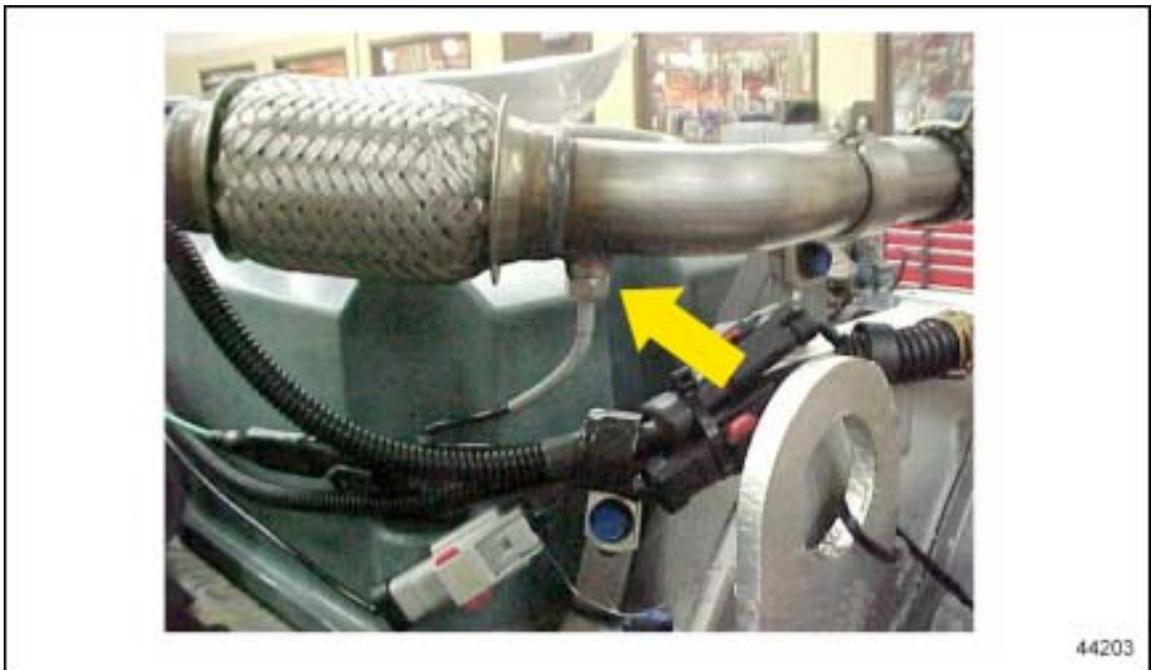
**Figure 2-13 EGR Temperature Sensor**
