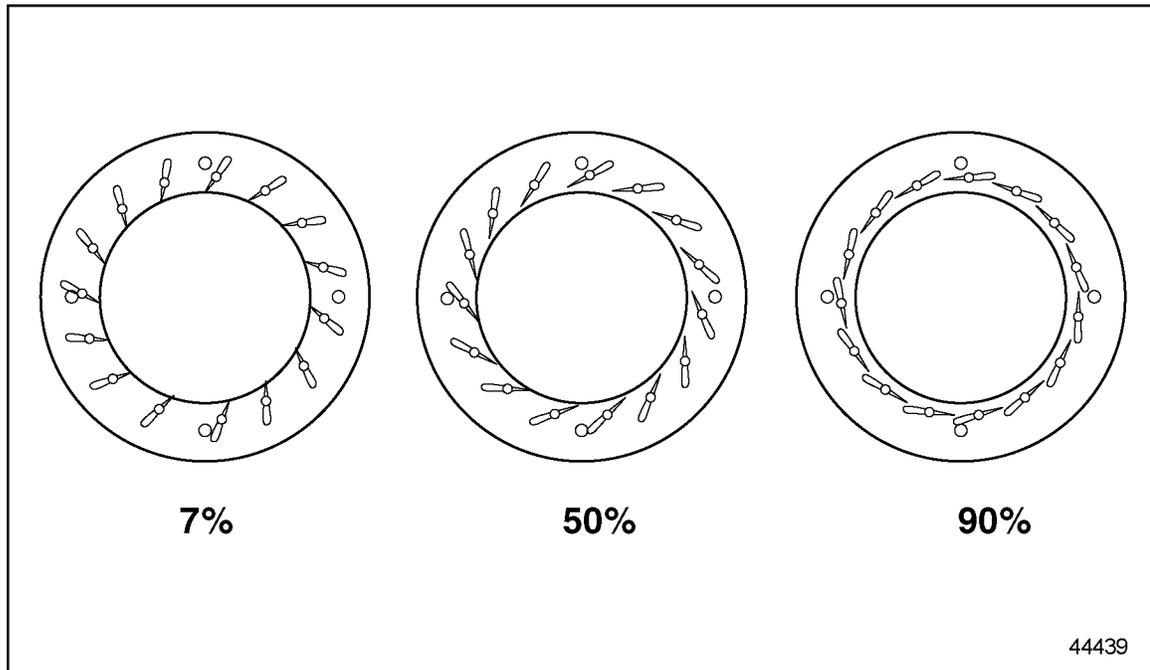
**Figure 2-7 VNT Vane Position**
