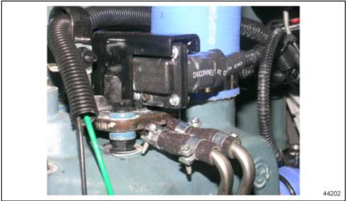
**Figure 2-12 Delta Pressure Sensor**
