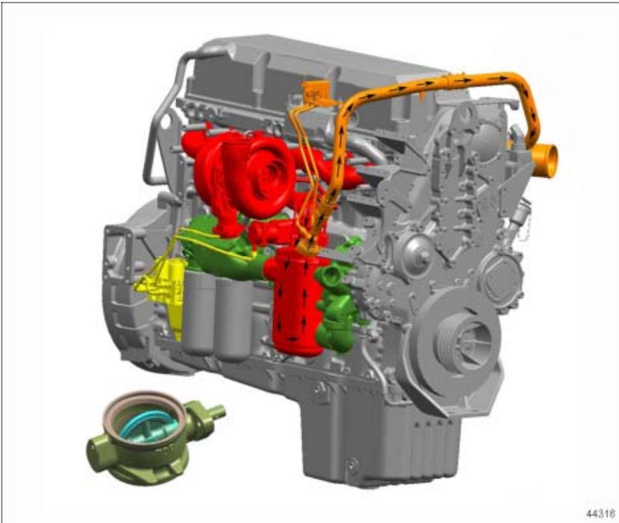
Air pressure supplied by the EGR VPOD to the EGR actuator opens the butterfly valve. Once the EGR butterfly valve opens, the EGR flows through the EGR cooler and into the delivery pipe.
