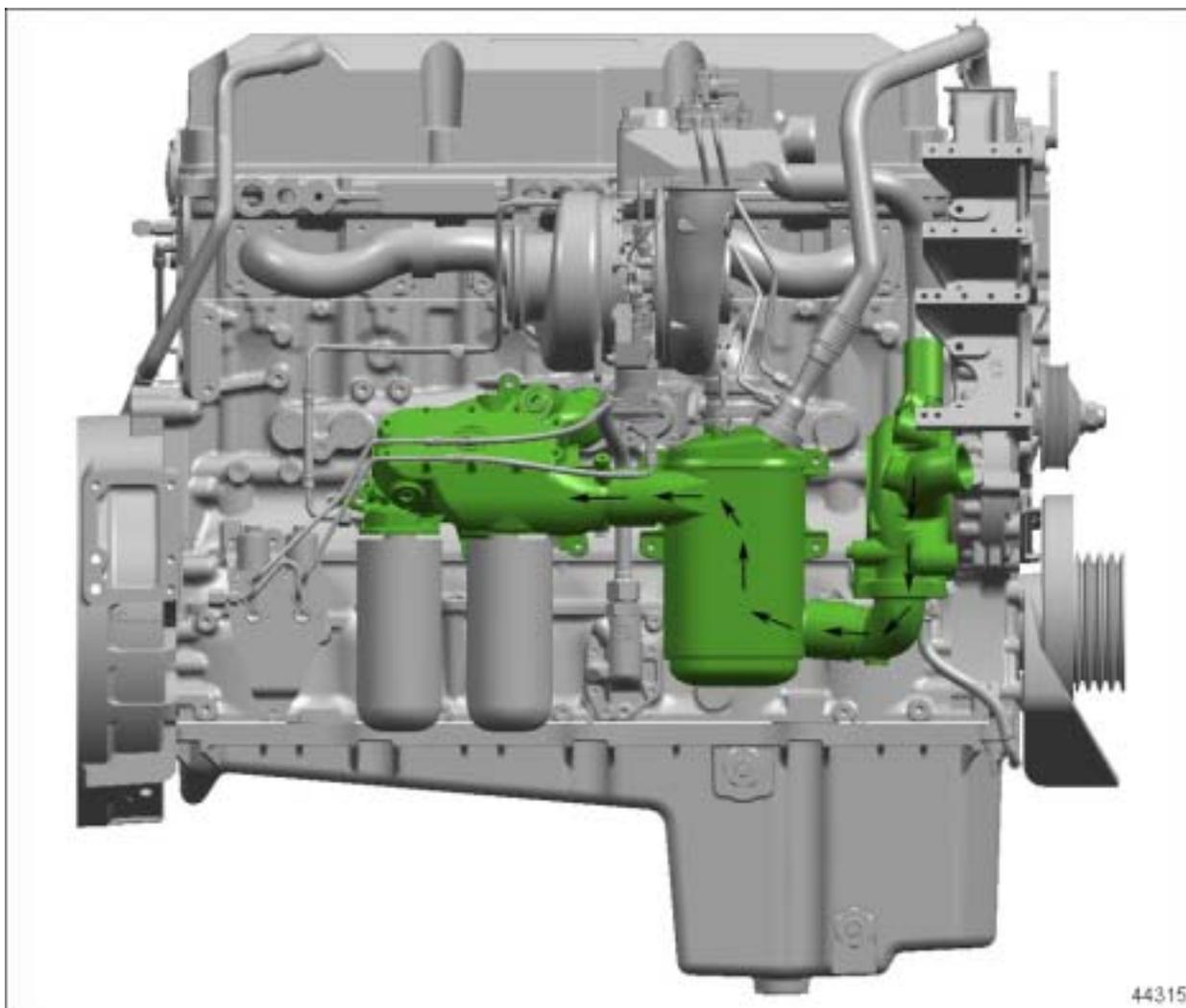
Exhaust gas enters the EGR cooler at high temperatures and is cooled by the engine coolant system to increase the density of the gas. **This graphic illustrates coolant flow.**
