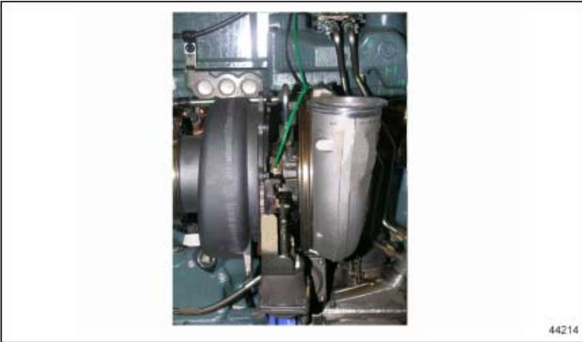
**Figure 2-5** VNT Turbocharger
