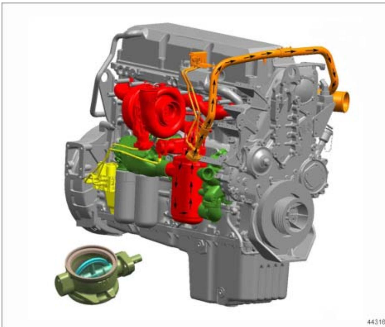
The VNT turbocharger is the mechanism used to change the EGR rate.
