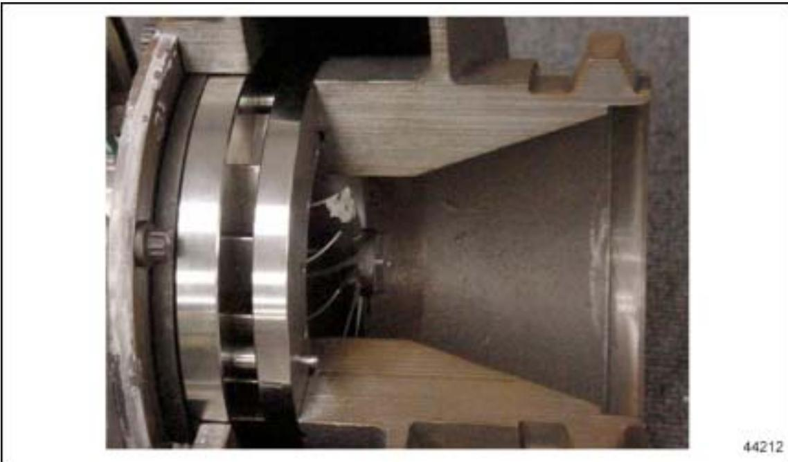
**Figure 2-6** Cut Away View of the Vanes
