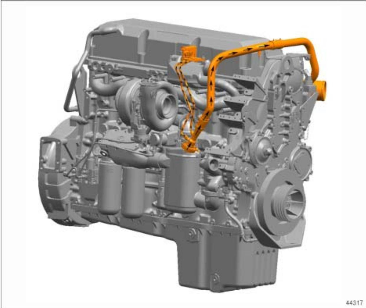
Once EGR begins flow through the EGR cooler and past the venturi, pressure levels are measured from the two venturi taps or ports. The delta pressure measurement, in conjunction with the EGR temperature, determines the EGR flow rate.
