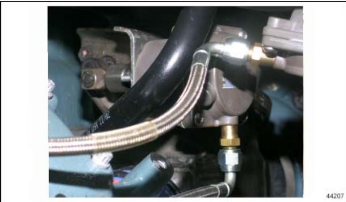
**Figure 2-8 EGR Valve Actuator**
