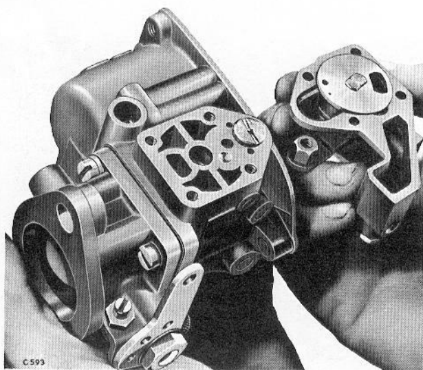
Fig. 35. Removing bi-starter from carburettor
