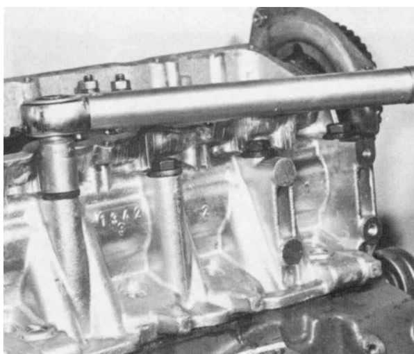
3.62A Tighten the cylinder head bolts and nuts to the specified torque
