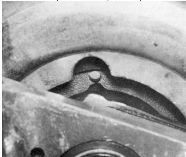
3.59 Hole in pulley aligned with část ridge, view from behind the wheel
