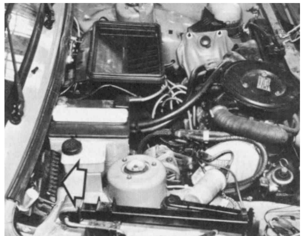
7.6 Location of fuse block - 1049 cc engine models
