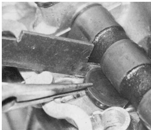
3.88B ...the shim can be removed
