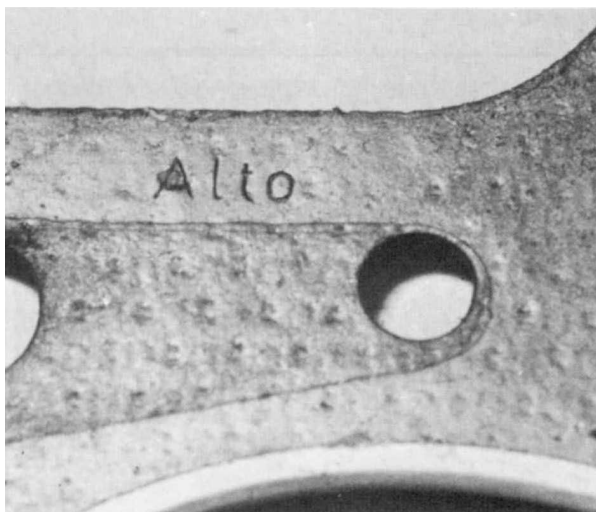
3.60 The cylinder head gasket is fitted ALTO upwards
