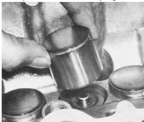
3.49D Refit each tappet bucket with its shim to its valve
