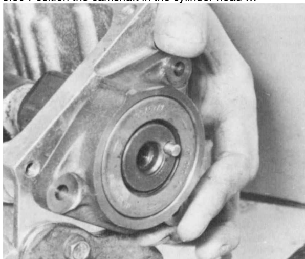
3.53 Fit the camshaft seal in its carrier to the cylinder head.
