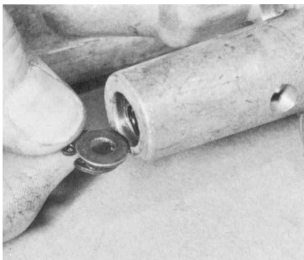
3.27B ...followed by the retainer plate and circlip
