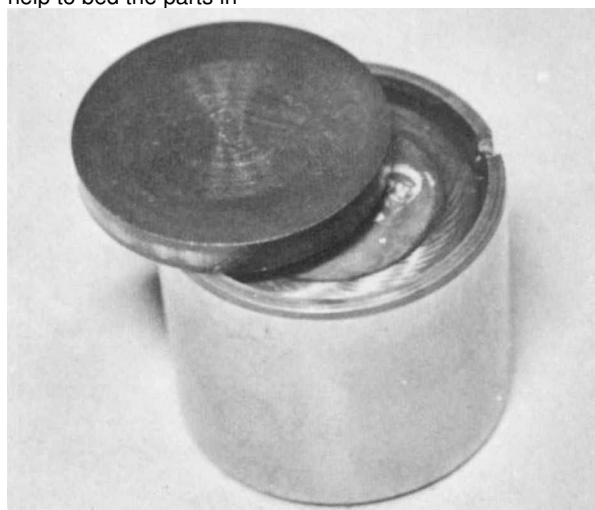
3.49B ...prise out the valve clearance adjusting shim
