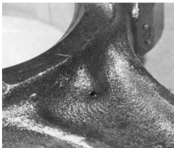
3.17 One of the oil jet holes in the big-end – the other is on the other side of the rod
