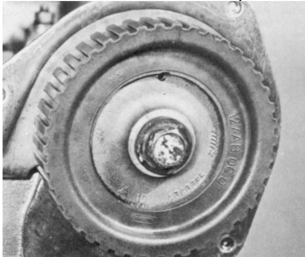
3.56 Fit the camshaft toothed pulley
