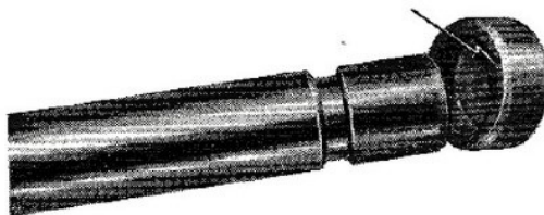
Fig. 35. - Detail of a valve stem and different thickness cups for clearance adjustment.
