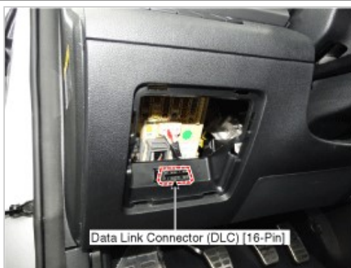
30. Data Link Connector (DLC) [16-Pin]
