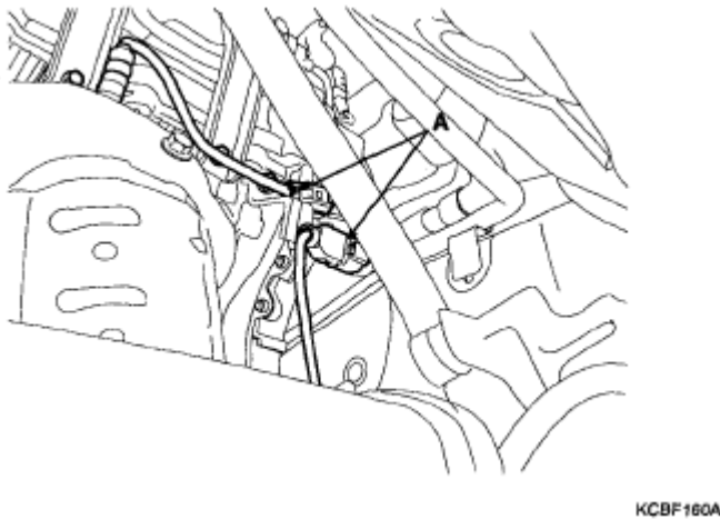
Fig. 125: Disconnecting Bank 1 Front/Rear O2 Sensor Connectors Courtesy of HYUNDAI MOTOR CO.
