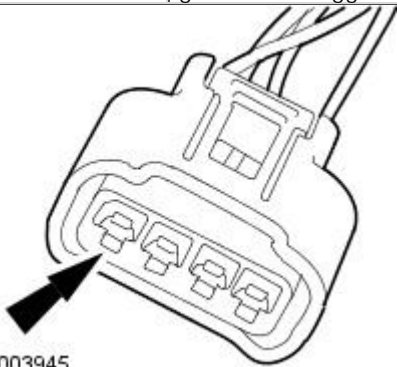
1B, 2B, 3B Ignition Coil Harness Electrical Connectors
