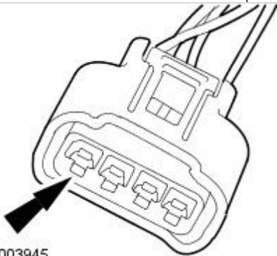
1A, 2A, 3A Ignition Coil Harness Electrical Connectors
