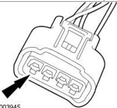
1A, 2A, 3A, 4A Ignition Coil Harness Electrical Connectors
