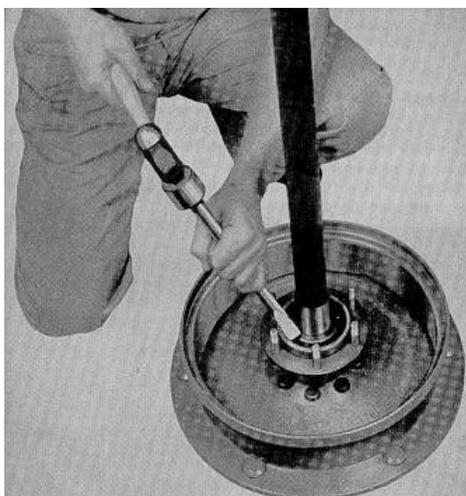
Fig. F068 - Removing the shrunk-on wheel axle shaft bearing retainer collar.
