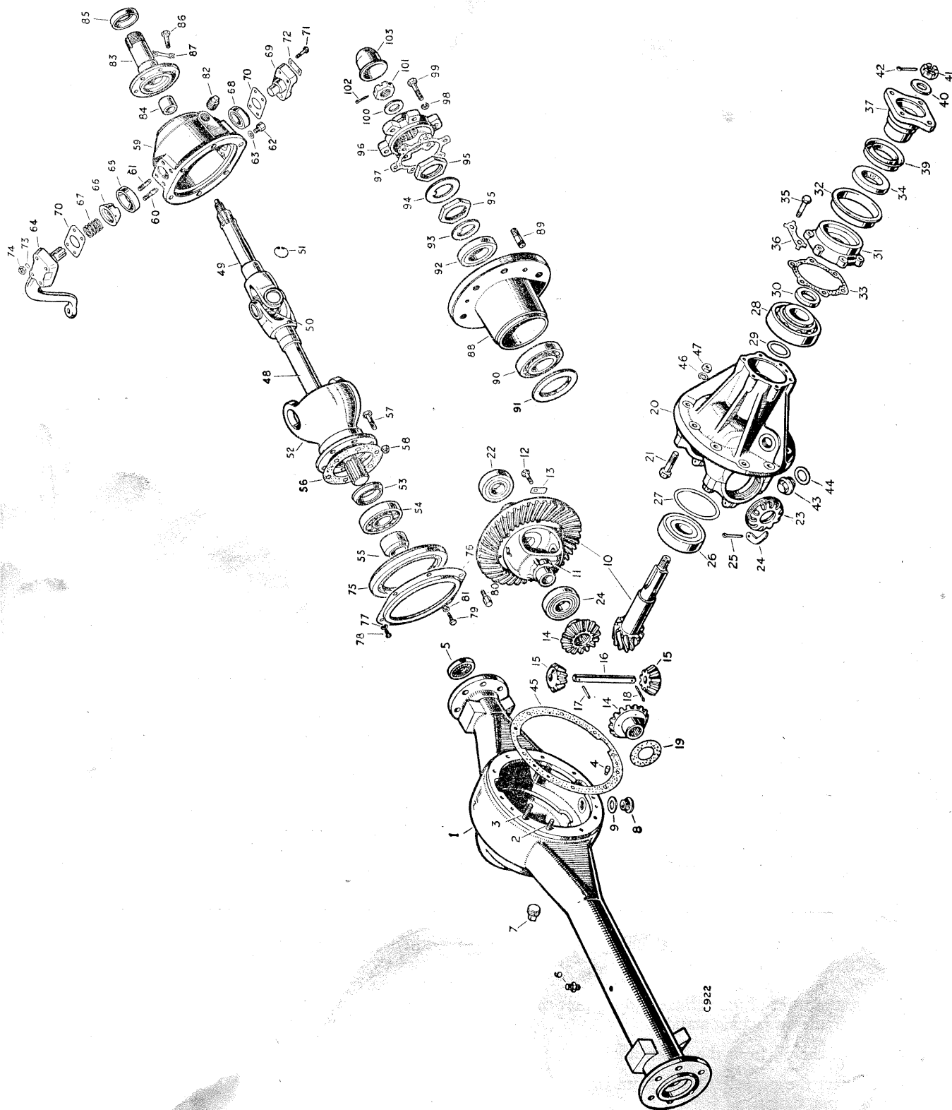
Fig. F-1—Layout of front axle
