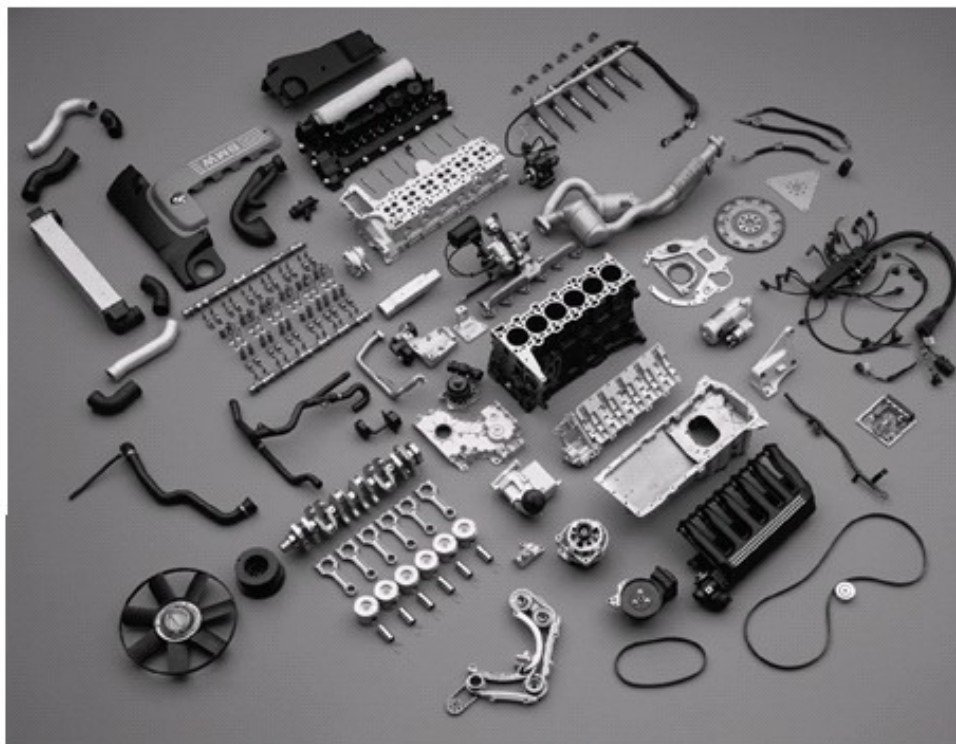
Fig. 10: Engine components and add-on parts - M57
