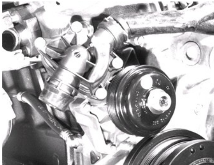
Fig. 47: Water pump - M57
