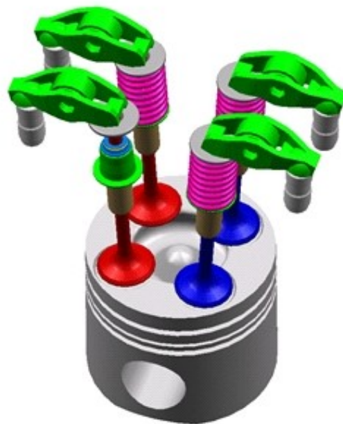
Fig. 19: Valve gear - M47/M57/M67
