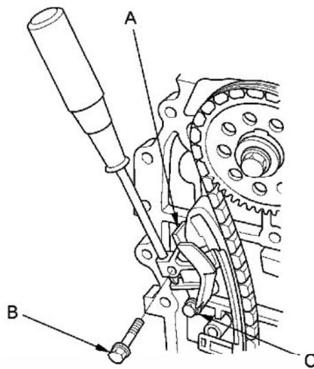
15. Hold the cam chain tensioner slider with the screwdriver, then remove the bolt (B), and loosen the bolt (C).
