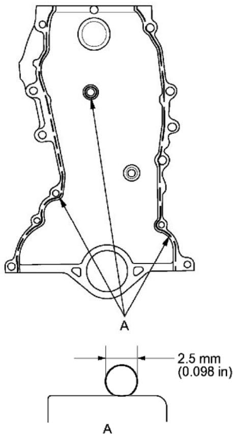
14. Apply liquid gasket (P/N 08717-0004, 08718-0003, or 08718-0009) to the oil pan mating surface of the cam chain case and to the inside edge of the bolt holes. Install the component within 5 minutes of applying the liquid gasket.
