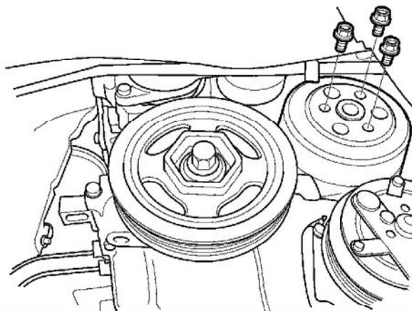
8. Remove the crankshaft pulley See: Cylinder Block Assembly/Harmonic Balancer - Crankshaft Pulley/Service and Repair.
