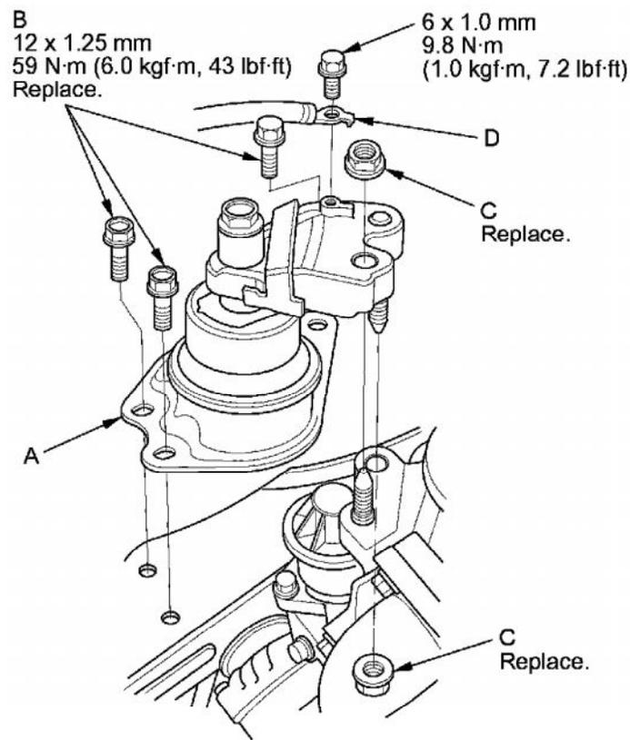
18. Loosely tighten the new side engine mount/bracket assembly mounting nuts (C).
