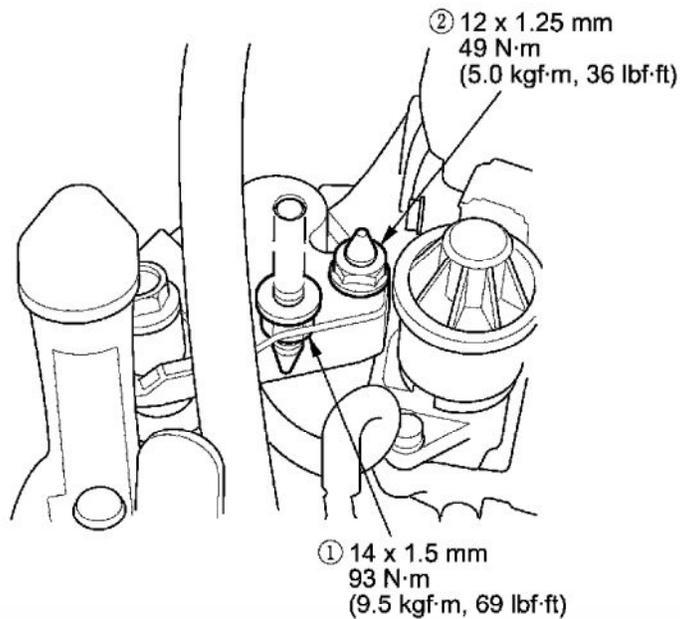
26. Tighten the transmission mount mounting bolts and nuts in the numbered sequence shown.
