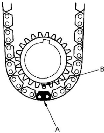
5. Install the cam chain on the camshaft sprocket with the pointers (A) aligned with the three colored pieces (B) as shown.
