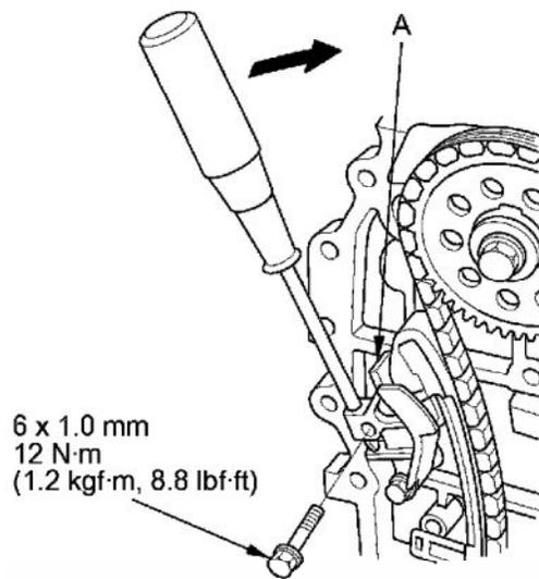
9. Rotate the cam chain tensioner slider clockwise to compress the cam chain tensioner, and install the remaining bolt, then tighten the bolts.
