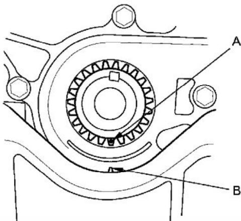
2. Remove the crankshaft sprocket.
