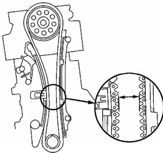
14. Apply new engine oil to the sliding surface of the cam chain tensioner slider (A).
