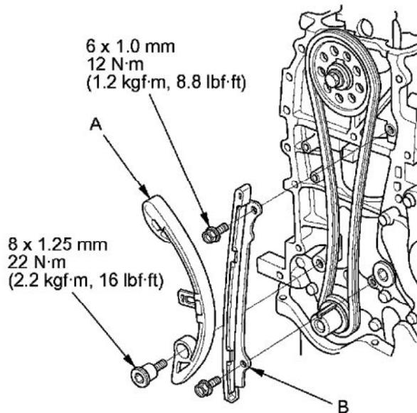
7. Install the cam chain tensioner slider, and loosely tighten the bolt.
