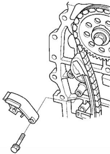
8. Apply new engine oil to the sliding surface of the cam chain tensioner slider (A).
