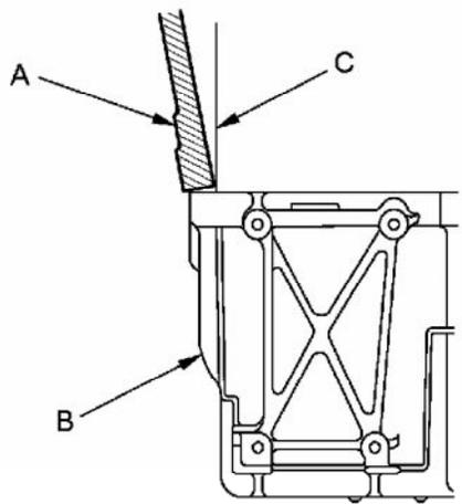
16. Tighten the chain case mounting bolts. Wipe off the excess liquid gasket on the oil pan and the chain case mating area.
