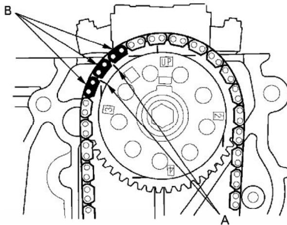
6. Install the cam chain tensioner (A) and the cam chain guide (B).
