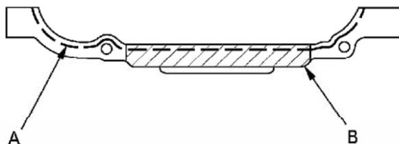
15. Set the edge of the chain case (A) to the edge of the oil pan (B), then install the chain case on the engine block (C).
