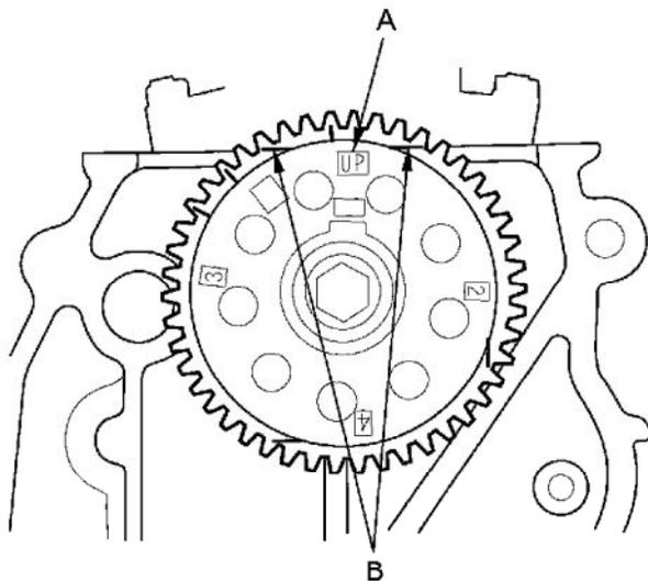
4. Install the cam chain on the crankshaft sprocket with the colored piece (A) aligned with the TDC mark (B) on the crankshaft sprocket, then install the crankshaft sprocket to the crankshaft.
