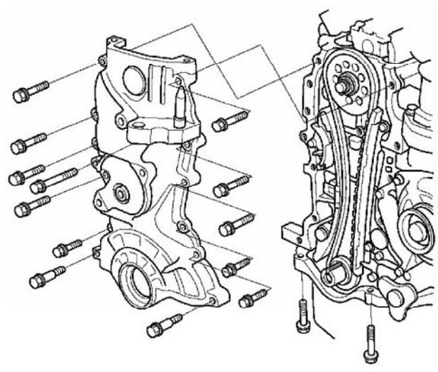
13. Measure the cam chain separation. If the distance is less than the service limit, replace the cam chain and cam chain tensioner.
