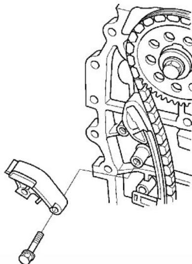
17. Remove the cam chain tensioner (A) and the cam chain guide (B).
