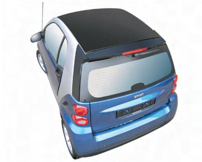
Vehicle with PU roof
