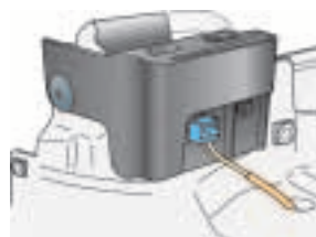
Left tonneau cover switch F348
