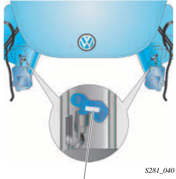
Early crash sensors in longitudinal member
