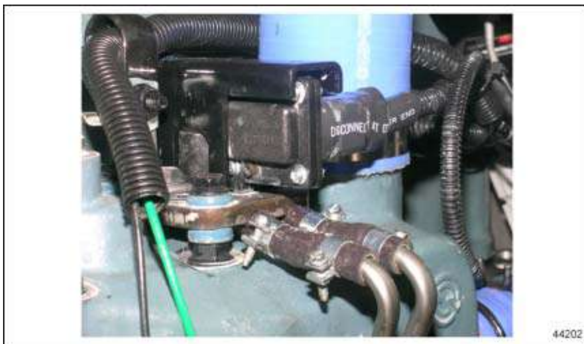
Figure 2-12 Delta Pressure Sensor
