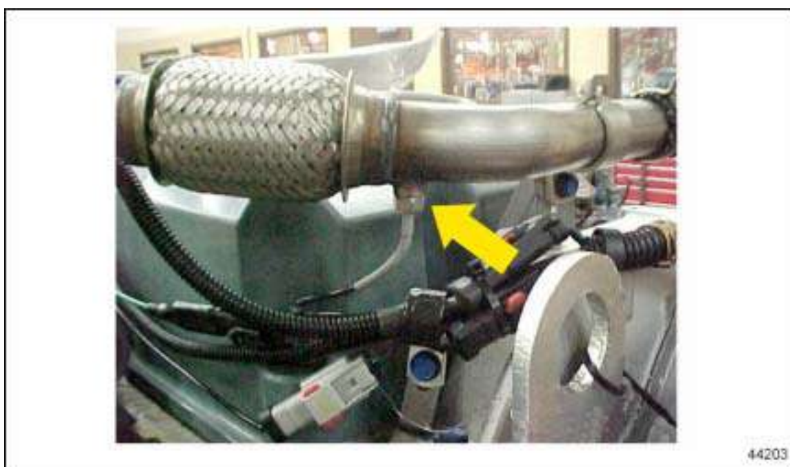
Figure 2-13 EGR Temperature Sensor
