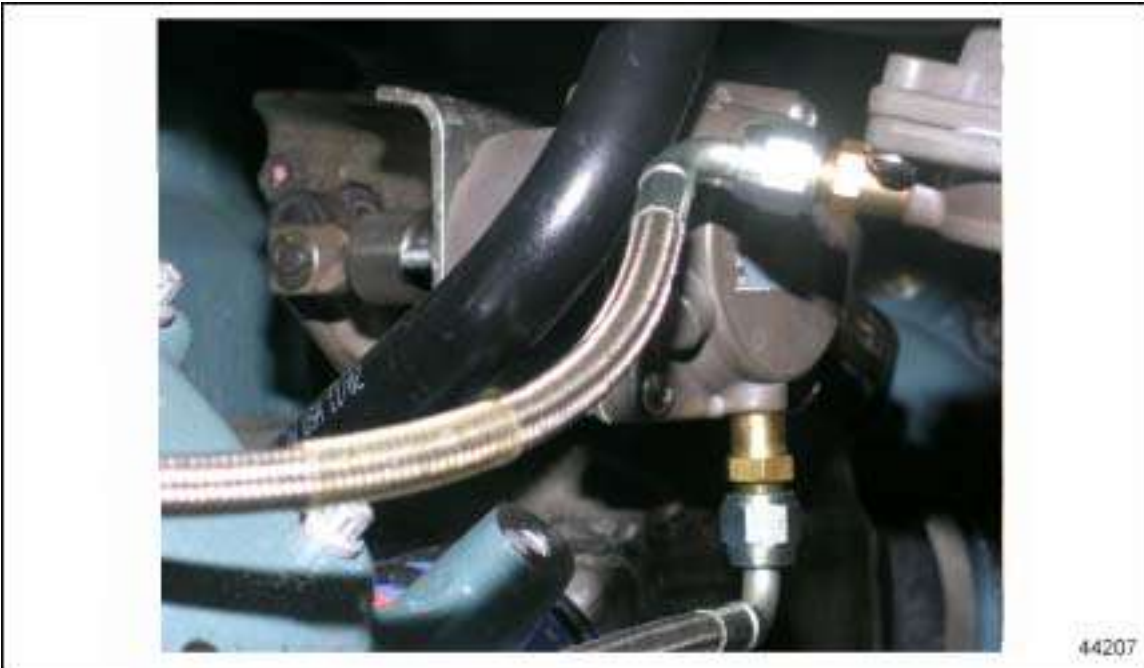
Figure 2-8 EGR Valve Actuator
