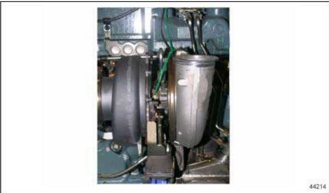
Figure 2-5 VNT Turbocharger
