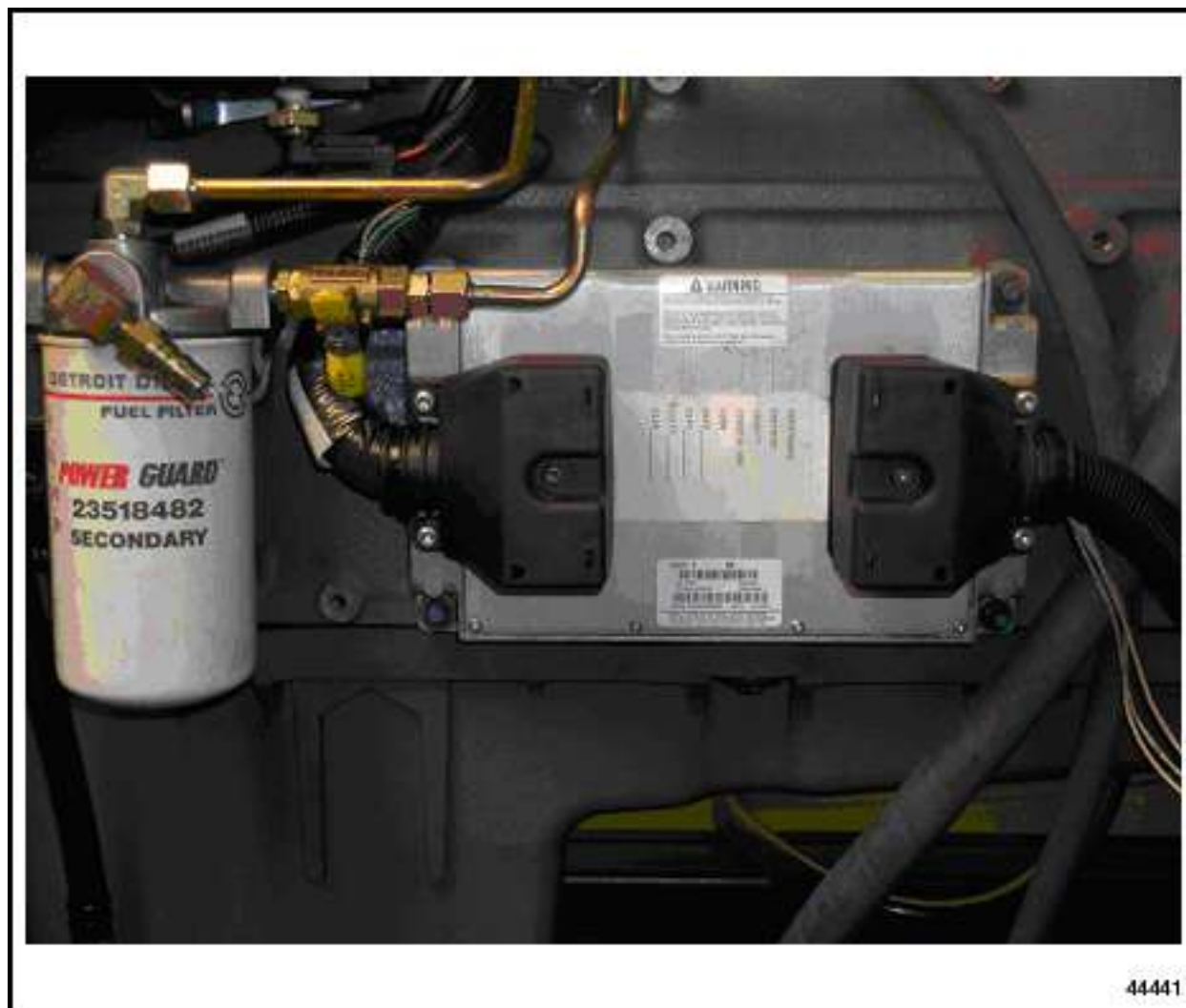
Figure 8-1 DDEC V ECU
