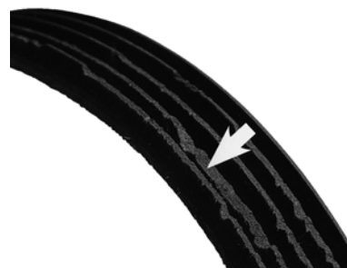
UNEVEN RIB WEAR
