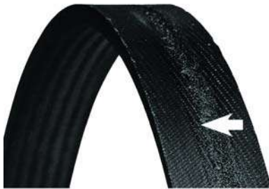
IMPROPER INSTALL
