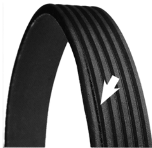
IMPROPER INSTALL
