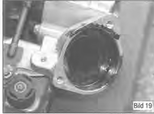
Fig. 19 Oil-smeared charge-air system: Stubborn oil deposits can be caused by a worn or damaged supercharger. This must be investigated.
