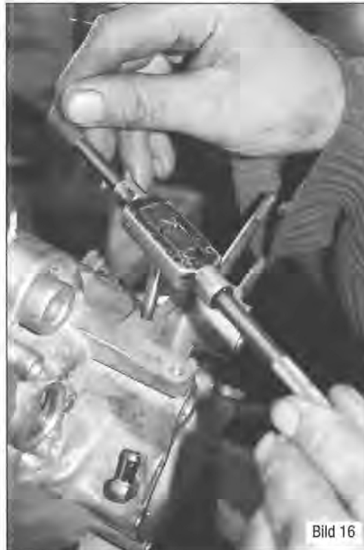
Image16 Thread cutting with care and consideration.
