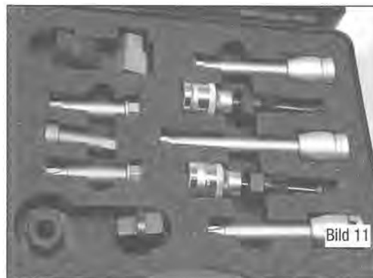
Figure 11 Disassembly kit for generator freewheels of different manufacturers: Different inserts for the freewheel hub and the alternator shaft enable removal even with different alternator manufacturers. m
