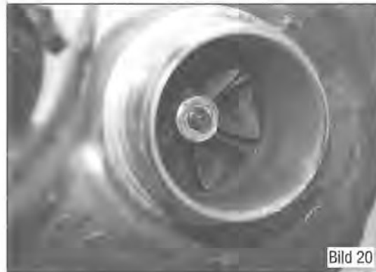
Fig. 20 Compressor Noise and oil loss are the first signs. This damage was discovered just in time. The nut of the compressor impeller had run on and was found in the charge-air chamber. coolL. ader total damage. en
