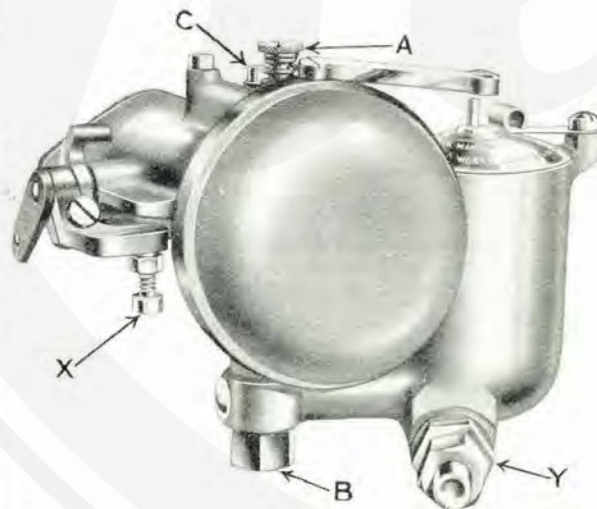
Fig. 7. The Smith Single-jet Carburetter.
