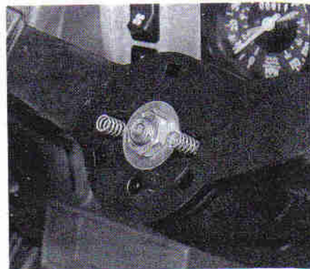
7.9 Make sure the springs fit inside the guide recesses
