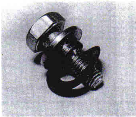
4.10B Maintain the correct assembly order of the bolt, collar and washer
