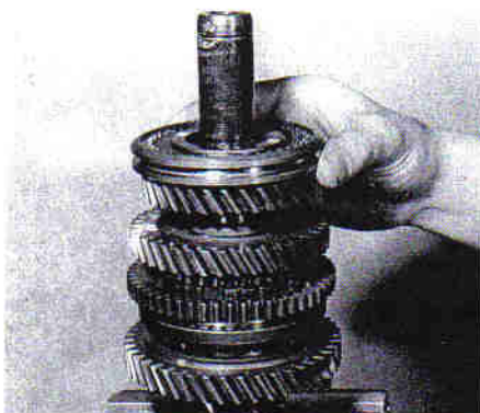
8.14 Fitting 3rd gear and synchroniser sleeve
