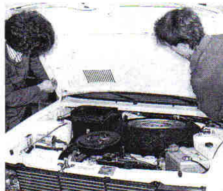
7.4 Lifting off the bonnet on a 45A model
