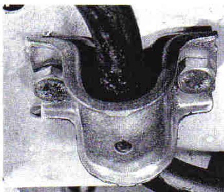
7.2 Anti-roll bar-to-body bracket
