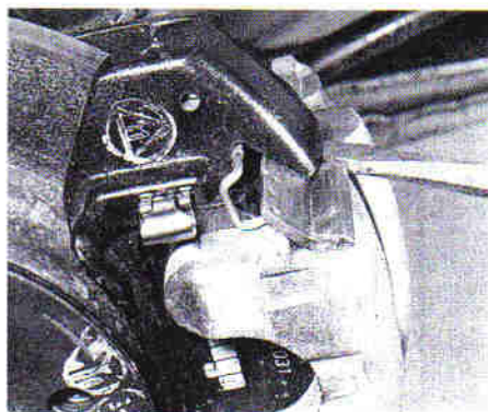
4.3B ... and slide out the locking blocks
