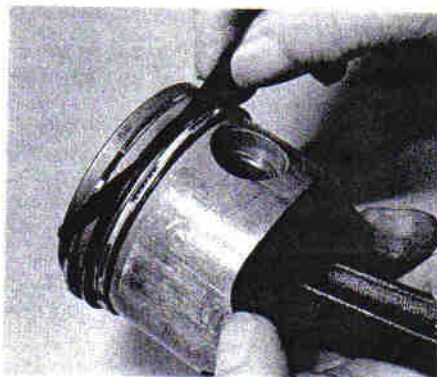
18.24A Checking piston ring groove clearance ...
