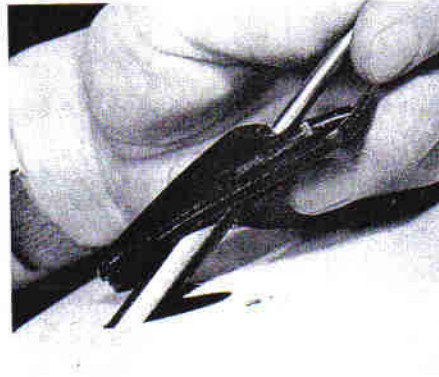
39.6 Withdrawing the aerial from the 'A' pillar
