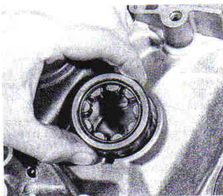
6.4 Lifting out the mainshaft bearing from the bellhousing
