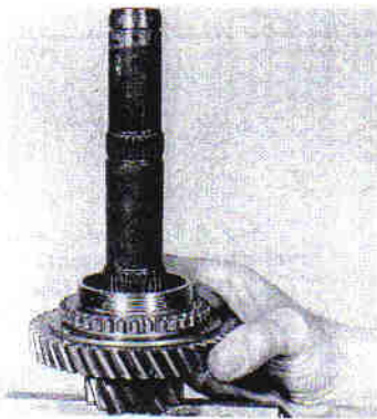
8.8 Fitting 1st gear ...
