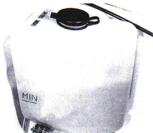
4.10B 'MIN' mark on 45/55/65 model expansion tank ...
