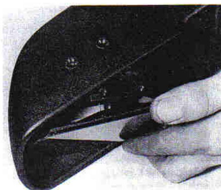
22.13B ... and withdraw the mirror glass ...
