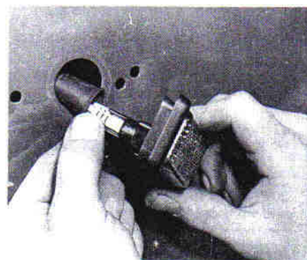
18.2A Removing the side repeater light on a 3/4/5 series model
