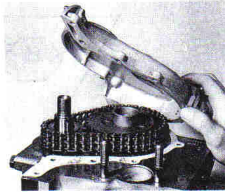
6.21 ... and the timing gear cover
