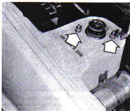
3.3A Suspension strut top mounting nuts on a 45 model ...
