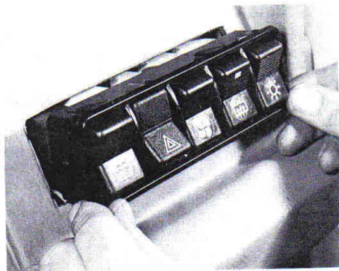
26.2 Removing a control switch assembly from the facia
