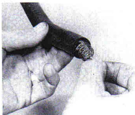
21.9 Removing the flame trap from crankcase breather hose
