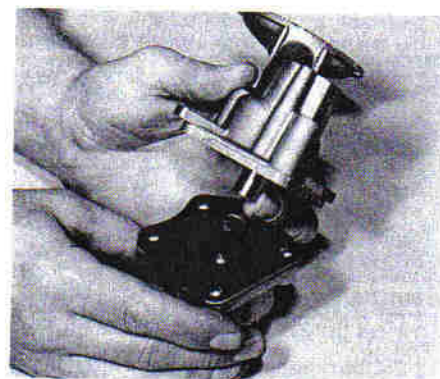
18.45 Separating the oil pump halves
