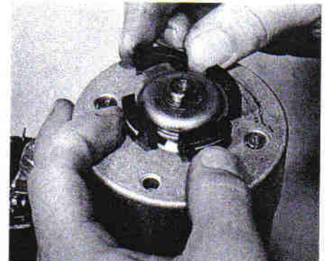
12.6 Remove the four carbon segments
