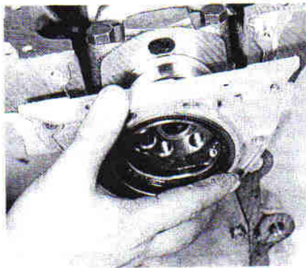
42.7B Fitting the rear crankshaft oil seal housing
