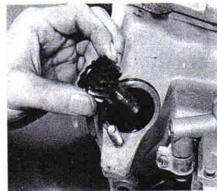
42.16 Fitting the distributor/oil pump drivegear
