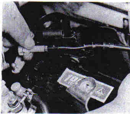
7.3 Releasing the cable from the bracket on the valve cover
