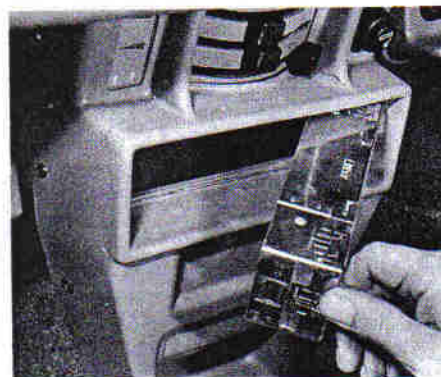
38.7 Removing the metal frame from the console
