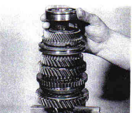
8.18 Fitting the bearing over the end of the shaft
