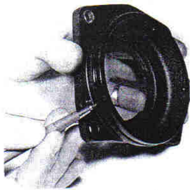
6.9C Removing the O-ring seal
