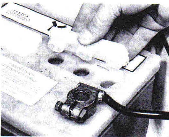
3.4 Triple unit plug being removed from battery
