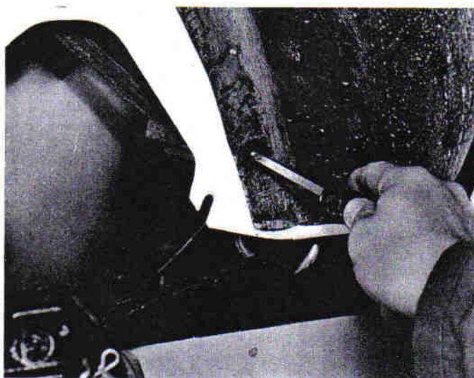
39.2 Unscrewing a wheel arch panel securing plug
