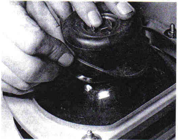
14.3 Peel back the rubber cover
