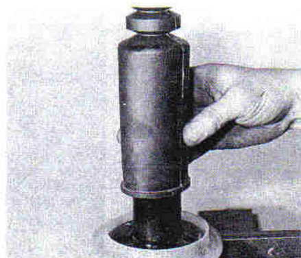
4.16 Slide on the rubber cover
