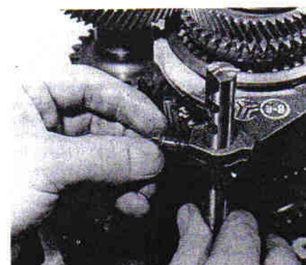
9.11A Fitting a selector fork lockbolt
