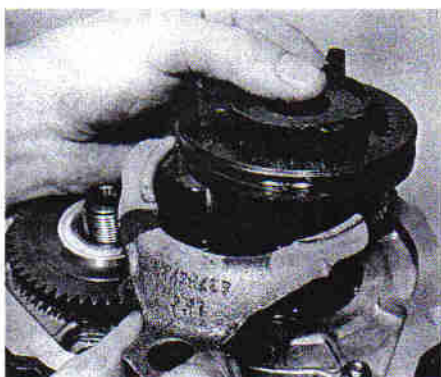
9.29A Fitting the 5th gear synchroniser assembly and selector fork
