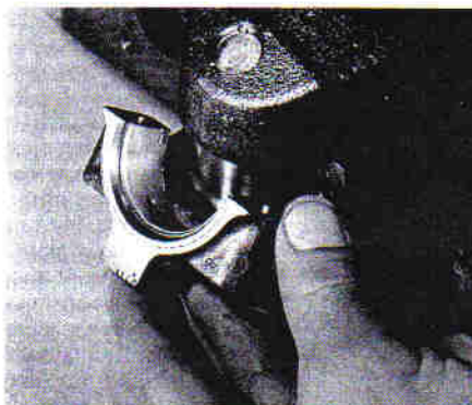
9.23 Fitting bearing cap to connecting rod
