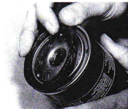
3.8 Fitting sealing ring to oil filter
