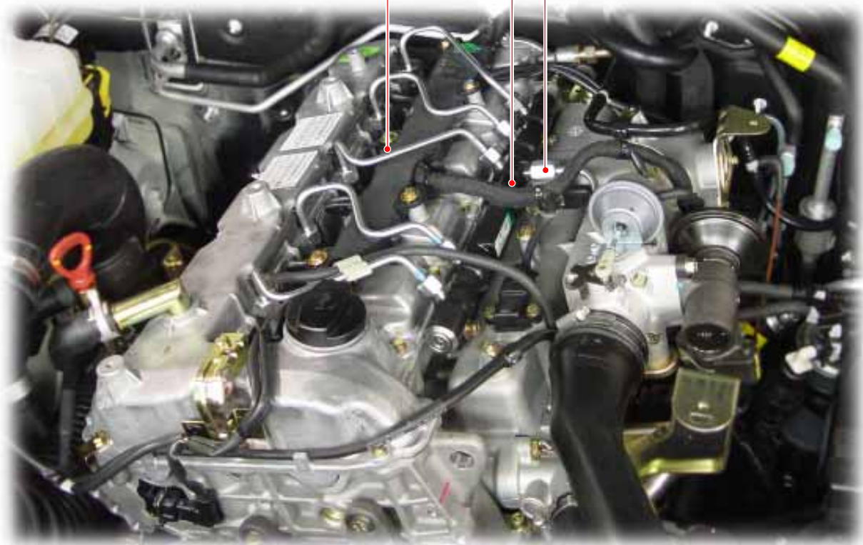
Fuel Supply Pipe (HPP-Common Rail) : Increase in I.D and O.D
