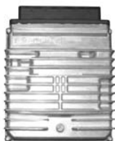
ECU/barometric sensor
