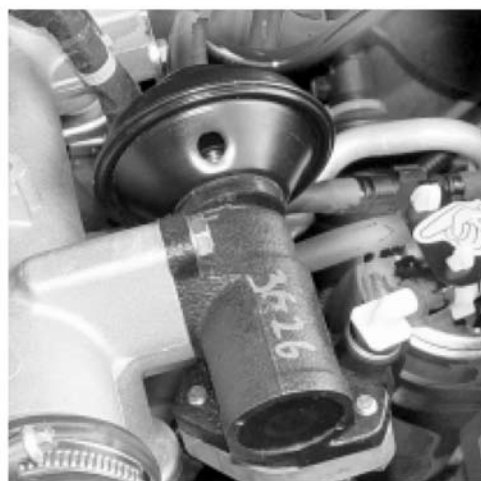
EGR System for DI Engine
