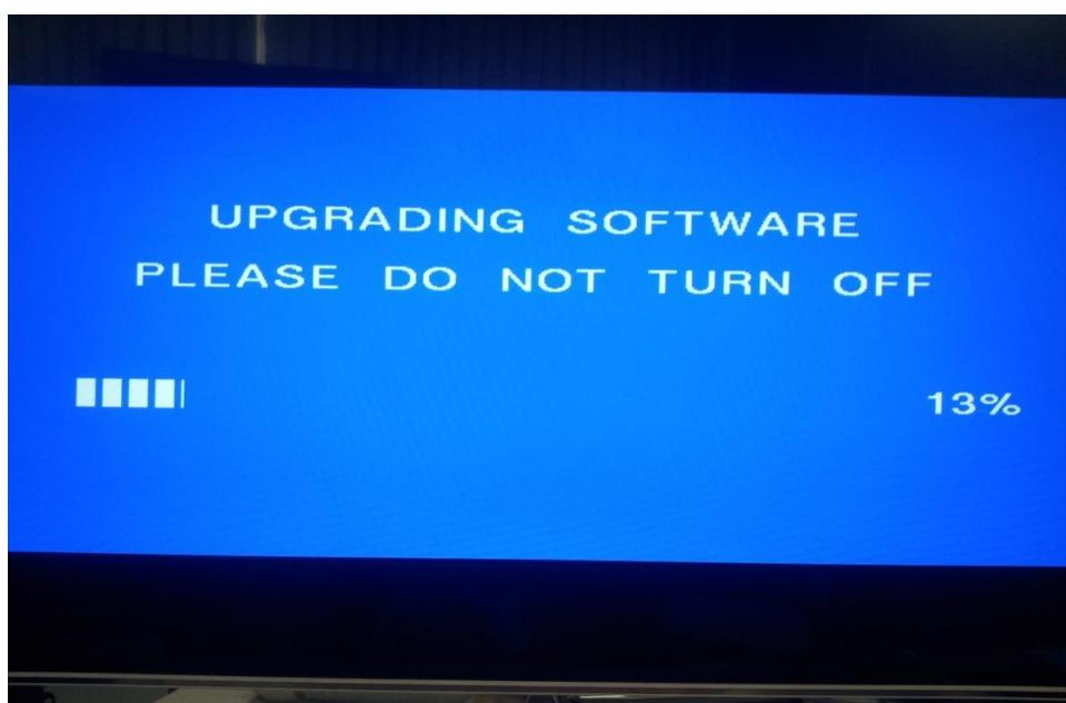
9、3). When update finished, TV will automatically shut down and then boot. Then Set default the TV: Setting--->Option->Restore Factory Default.
