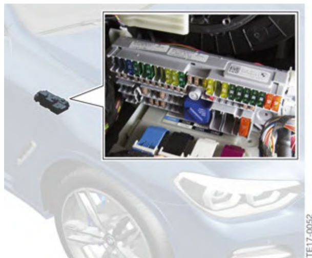
Power distribution box, front right
