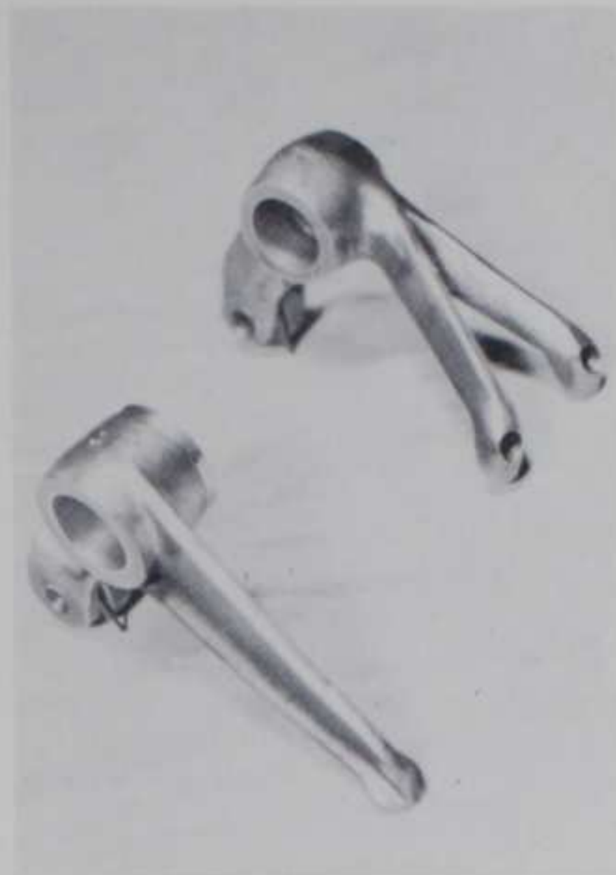
Right: Rocker arms—183 cu. in. racing engine
