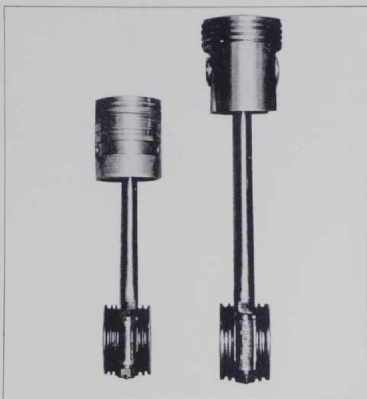
At the left is the piston and connecting rod assembly of the Duesenberg racing car, while the other is that of the stock car. Both rods are tubular and carry cooling flanges
