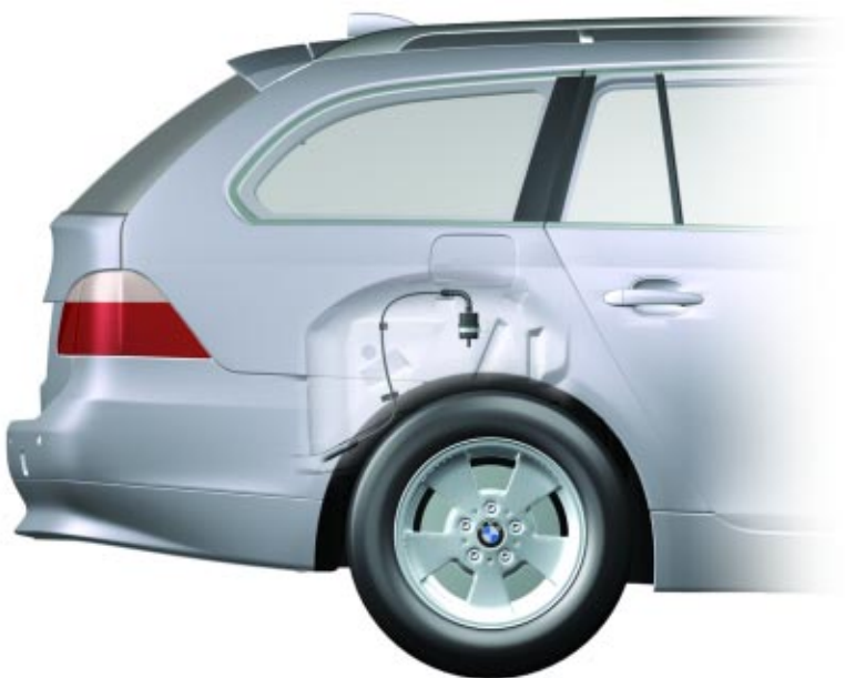
Location of air filter for LVA
