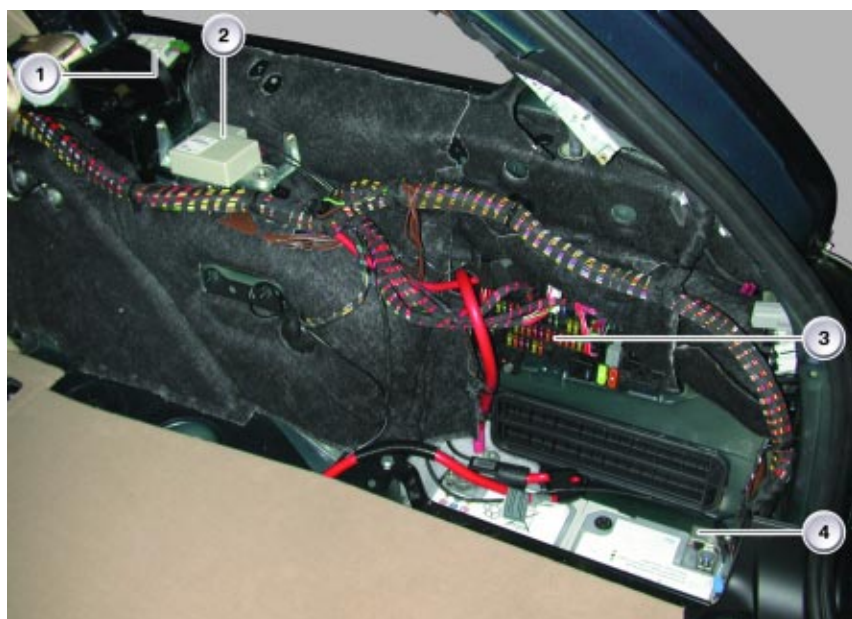
Control Units in Luggage Compartment, Right
