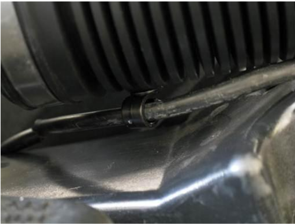
Install MAF electrical cable in clip under intake boot.
