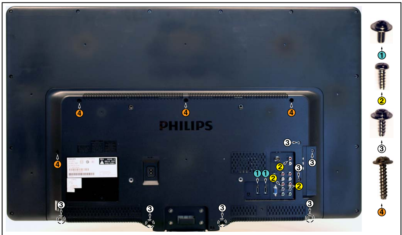
Figure 4-4 Rear cover removal (42")
