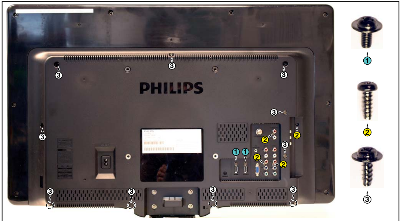
Figure 4-3 Rear cover removal (32")
