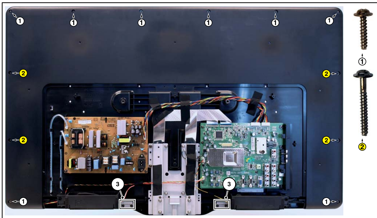
Figure 4-10 Bezel removal (42")
