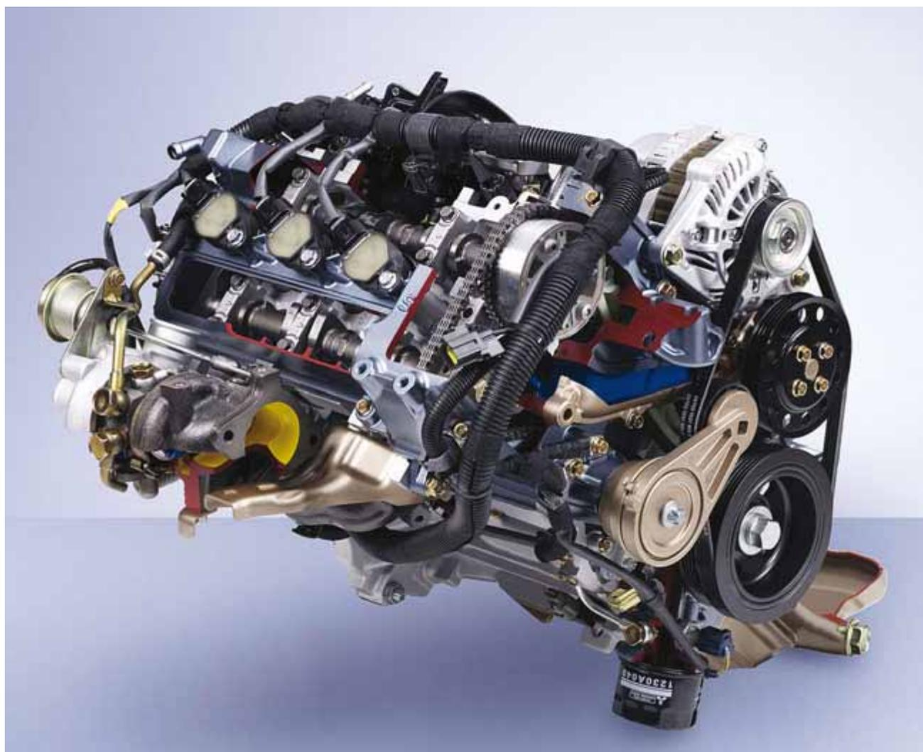
Shown on 3-cylinder gasoline engine with turbocharger
