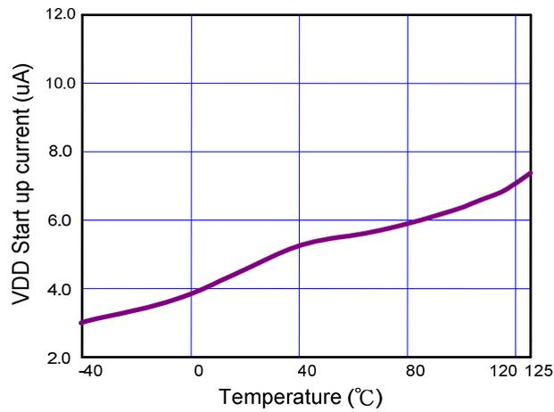
Fig. 1 VDD Start up current vs. Temperature
