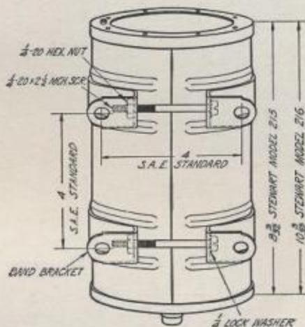
Fig. 4. Outside shell assembly, showing brackets. Bolts or screws to fit the holes in brackets can be  $\frac{1}{2}$ " or  $\frac{3}{8}$ ";  $\frac{1}{2}$ " preferable.
