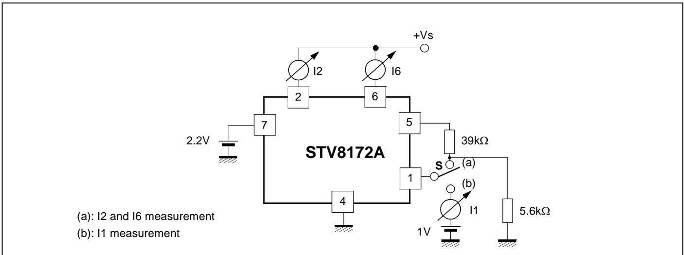
Figure 2: Measurement of  $V_{5H}$
