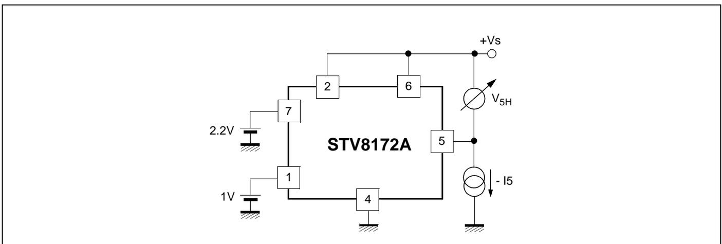
Figure 3: Measurement of  $V_{3L}$  and  $V_{5L}$
